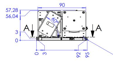
2 x M2.5x0.45 SCREWLOCK HELICOIL Insert = 1.0 \* Dia. Identical pattern opposite side Torque in Nm: First time on 0.97 First time off 0.75 Fifth time off 0.72
