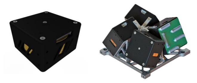
The wheel can be purchased as either single wheel without a mounting bracket or in a 4-wheel pyramid setup within a mounting bracket. The envelope of the reaction wheel is designed for allowing 4 wheels to be placed in a redundant setup within the envelope of a standard CubeSat.
