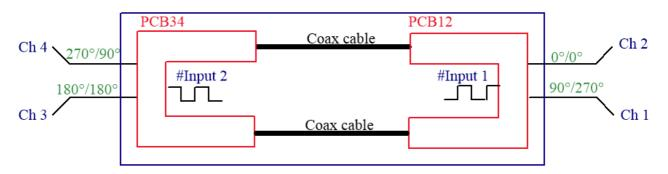
Figure 5 6U structure from the top, 2U side. Input signal at Input 1 or Input 2 and detection at Ch2, Ch1, Ch3 and Ch4. Green number are the expected phase of the received signal in degree at each channel. Each channel corresponds to an antenna rod.
