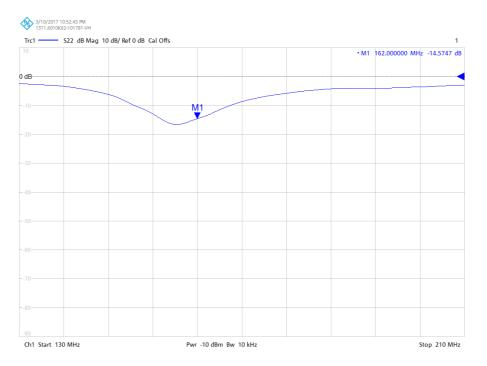
Figur 15 Return loss of one of the antenna ports with antenna rods and with matching components mounted on the other ports. Also, the full system installed on a 6U structure for more realistic results.
