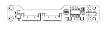
The front of the PCB contains all the electronics and connectors. The bottoms only contain the countersunk holes for mounting. Except for the antenna release, the whole PCB will be covered from the outside by solar panels.
