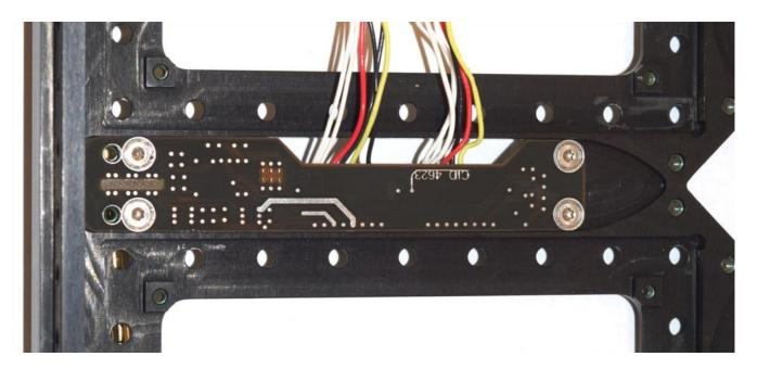
Bottom side shows the mounting with the countersunk screw holes
