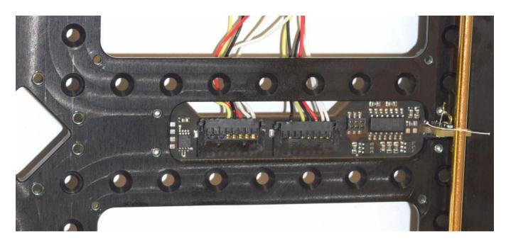
Top side with an antenna tied to the release mechanism and harnesses connected to show how the wires exit.
