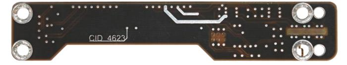
Contains no components. Four countersunk holes for M2 screws.
