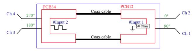
Figure 3 6U structure from the top, 2U side. Input signal at Input 1 and detection at Ch2, Ch1, Ch3 and Ch4. Green number are the expected phase of the received signal in degree at each channel. Each channel corresponds to an antenna rod.
