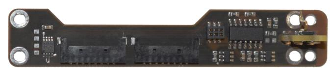
Components from left to right. I<sup>2</sup>C isolator, 2x Molex connectors, MCU connector, the MCU and the antenna release system.
